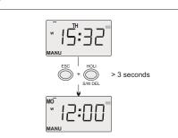
Besides the basic settings shown here, the two switching times stated in B2 are preset. Repeat the steps for initial operation
