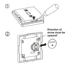
Note: The transmitter's coding is preserved even if there is no voltage supply. You do not need to re-register the code with the wireless control after a battery change.
