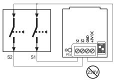
Transmission lasts as long as a connected button is pressed but max. 36 seconds.
