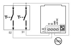
The transmission starts on every change of state of a connected switch and lasts approx. 0.5 seconds.
